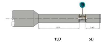
If there is a diverging tube with more than 15° located in the upstream, then the upstream straight  $\geq\! 18D$  , the downstream straight  $\geq\! 5D.$
