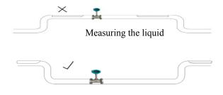
6. The installation of sensor on the vertical pipe
