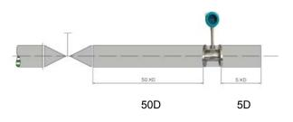
3.The upstream/downstream pipe of mounting point should be concentric with the sensor and the coaxial deviation should not be less than 0.5DN.
