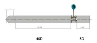
The valve should be installed at least 5D away from the downstream of sensor, if the valve must be installed on the upstream of sensor, the length of upstream straight pipe should not be  $\leq$  5D, the downstream should not be  $\leq$ 5D.
