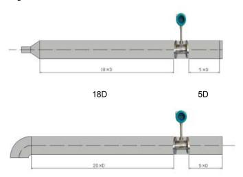
If there is a elbow or T-joint,with 90°,then the upstream straight  $\geq$  20D, the downstream straight  $\geq$  5D.
